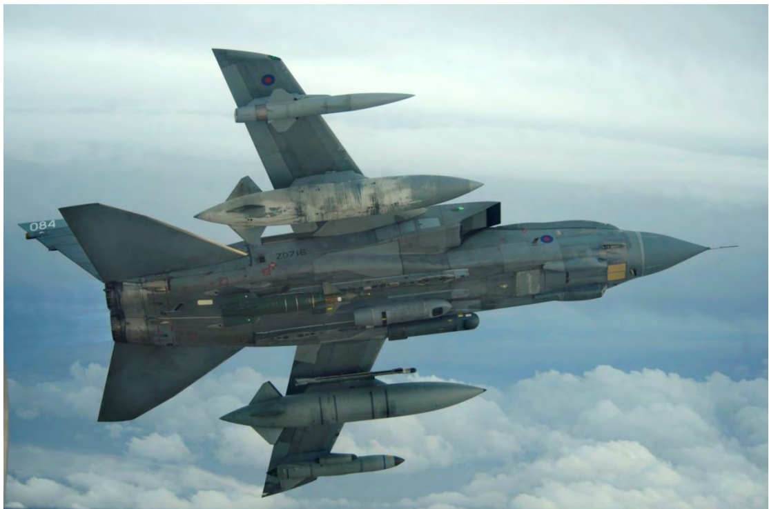
The Tornado GR.4 had replaced the Tornado GR.1 by the start of Operation Telic; this aircraft is carrying reconnaissance and targeting pods and a Paveway laser-guided bomb
